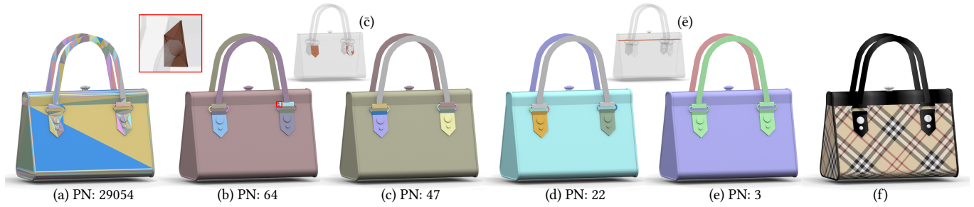
Fig. 3. The visual driven global mesh repair pipeline applied on a bag model from ShapeNet. From left to right: (a) the input mesh, with its scattered manifold surface patches (Sec. 4.1) rendered in different colors; (b) after preprocessing that merges coinciding vertices and removes duplicate faces (Sec. 3); (c) after visual-driven processing (Sec. 4) that further reorients and merges scattered patches and removes visually redundant patches shown in (c̄); (d) after the global optimization of patch orientation and connection (Sec. 5), intersecting patches (e.g. around the rings) are connected into coherent and larger pieces; (e) the global optimization applied on the subset of patches excluding hidden ones shown in (ē), to enable more connections of different components (Sec. 6.2); (f) is (e) rendered with textures copied from the initial input, which are well preserved by our minimally intrusive approach. The number of manifold surface patches PN is shown for each mesh. For (a) and (b), we have used two-sided shading so that their many flipped faces can be shown.
