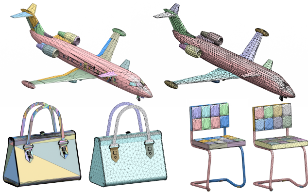
Fig. 12. Remeshing on the repaired models. For each pair, the left is the input model, and the right is our fixed model with each patch further remeshed by local operations like edge flipping and vertex smoothing [Fu et al. 2014]. Hidden patches are not removed here. Note that sharp curves on the input models are detected as feature lines and well preserved by remeshing.
